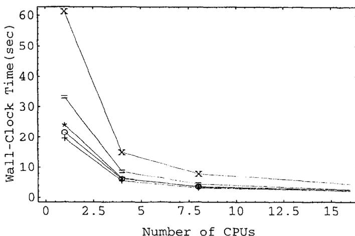
Fig. 5. Run-time for Problem 4 (Unpreconditioned). —x— (s,k)=(1,26), — — (s,k)=(2,1), —\*— (s,k)=(4,1), —+— (s,k)=(8,1), —o— (s)=(16,1).
