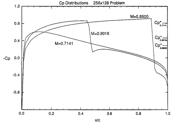
**FIG. 4.**  $C_p$  Distributions over NACA 0012 airfoil for cases tested on  $256 \times 128$  grid.
