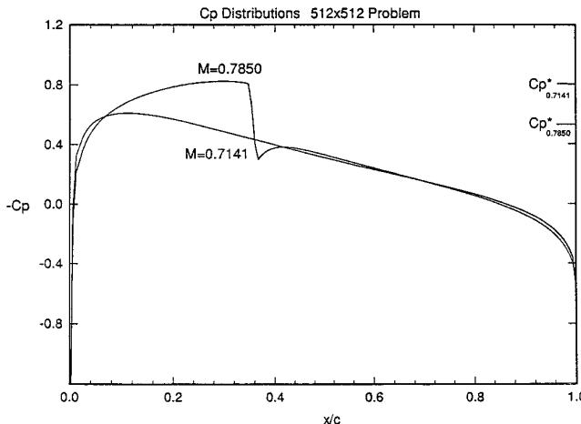
**FIG. 10.**  $C_p$  distributions over NACA 0012 airfoil for two cases tested on  $512 \times 512$  grid.
