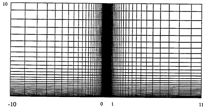
**FIG. 3.** Solution mesh ( $64 \times 32$  shown for illustration purposes, but actual meshes used are  $256 \times 128$  and  $512 \times 512$ ).
