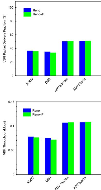
Fig. 12. VBR packet delivery fraction and throughput for the traffic consisting of 10 HTTP and 4 53-Kbps VBR connections with no background load from CBR sources.
