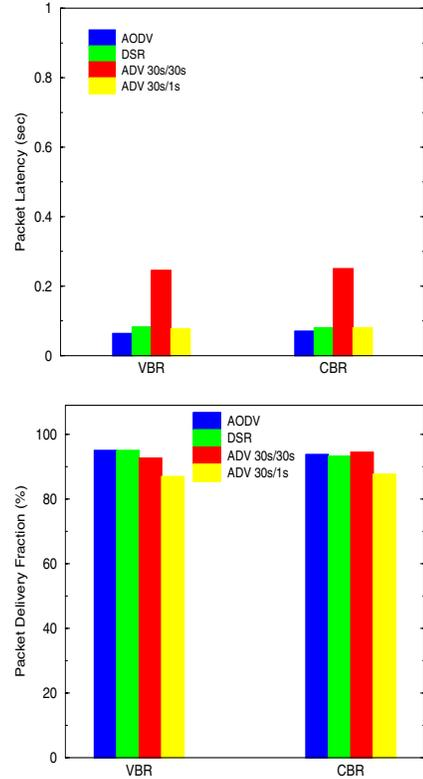
Fig. 6. Packet latency and delivery fraction for 10.6-Kbps VBR connections, and a 80-Kbps background load from 8 CBR sources.
