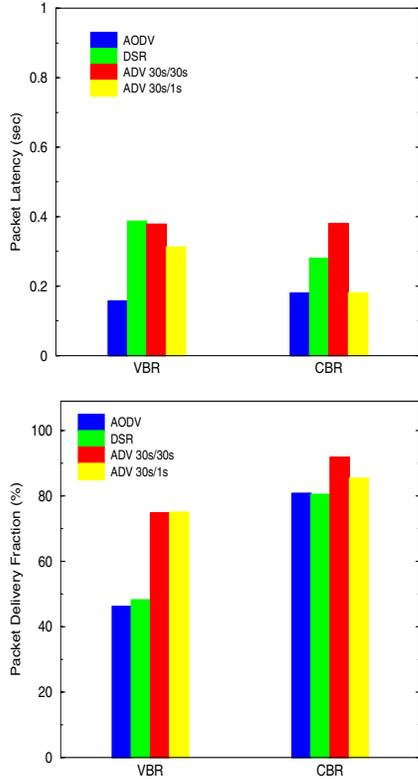
Fig. 5. Packet latency and delivery fraction for 2 53-Kbps VBR connections, and a 80-Kbps background load from 8 CBR sources.
