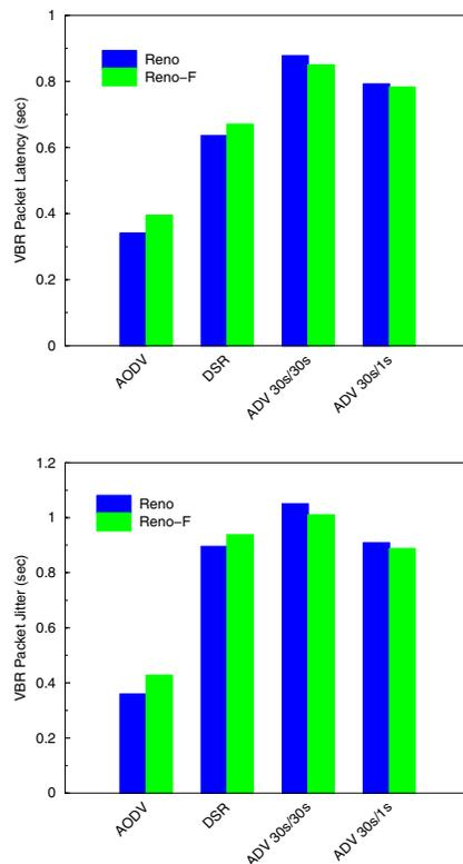
Fig. 8. VBR packet latency and jitter for the traffic consisting of 10 HTTP, 2 53-Kbps VBR connections, and a 80-Kbps background load from 8 CBR sources.
