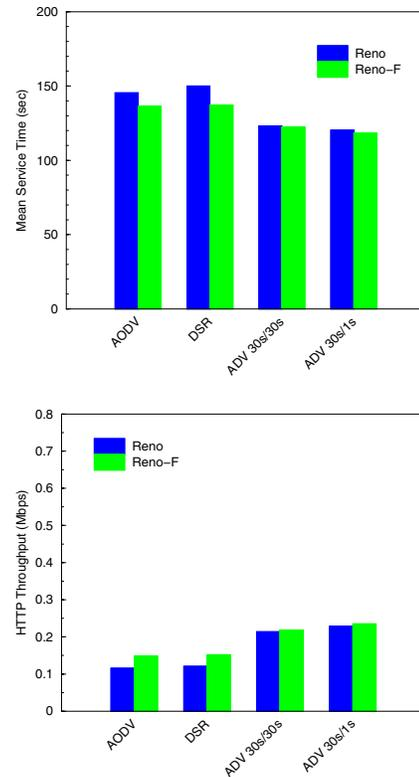
Fig. 10. Mean service time and throughput for the traffic consisting of 10 HTTP and 4 53-Kbps VBR connections with no background load from CBR sources.
