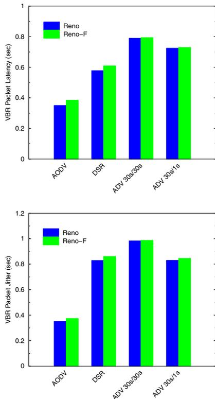
Fig. 11. VBR packet latency and jitter for the traffic consisting of 10 HTTP and 4 53-Kbps VBR connections with no background load from CBR sources.
