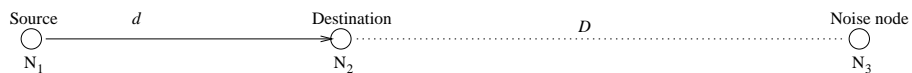
Figure A.1: Collision distance calculation. N_1 is the source and N_2 is the destination of the communication. N_3 is distant node whose transmission increases the noise level at N_2 .
