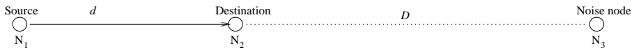
Figure 3.8: Collision distance experiment. N_1 is the source and N_2 is the destination of the communication. N_3 is a distant node whose transmission increases the noise level at N_2 .
