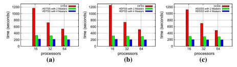
Fig. 9 The maximum difference in masters execution time for matrix multiplication using non-hierarchical distributed and hierarchical distributed schemes. **a** DTSS and HDTSS, **b** DFSS and HDFSS, **c** DGSS and HDGSS
