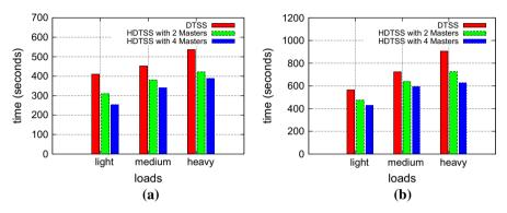
Fig. 12 The performance of hierarchical versus distributed schemes under varying loads. a QuickSort, b MatrixMultiply
