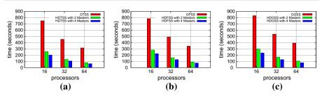
Fig. 8 The maximum difference in masters execution time for quick sort using non-hierarchical distributed and hierarchical distributed schemes. a DTSS and HDTSS, b DFSS and HDFSS, c DGSS and HDGSS
