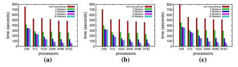
Fig. 3 The performance of adjoint convolution using hierarchical distributed schemes. **a** HDTSS, **b** HDFSS, **c** HDGSS
