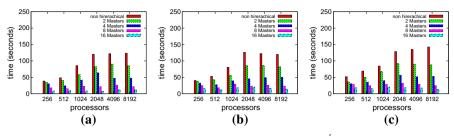
**Fig. 4** The non-overlapped communication and synchronization overhead  $T'_{overhead}$  of Mandelbrot set. **a** HDTSS, **b** HDFSS, **c** HDGSS
