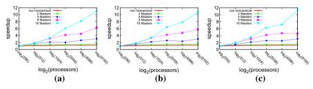
Fig. 6 The speedup of Mandelbrot set using hierarchical distributed schemes. a HDTSS, b HDFSS, c HDGSS
