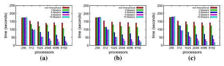
Fig. 2 The performance of Mandelbrot set using hierarchical distributed schemes. a HDTSS, b HDFSS, c HDGSS
