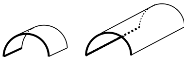
Figure 5: Combinatorially different Minkowski sums of a line segment and a circular arc.
