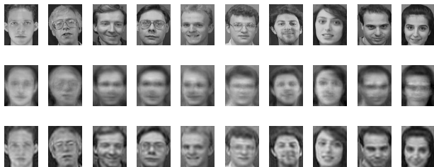
Figure 7: First row: raw images. Second row: images compressed by PCA. Third row: images compressed by GPCA.
