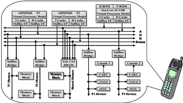
Figure 1: A Typical Virtual System Prototype for Mobility
