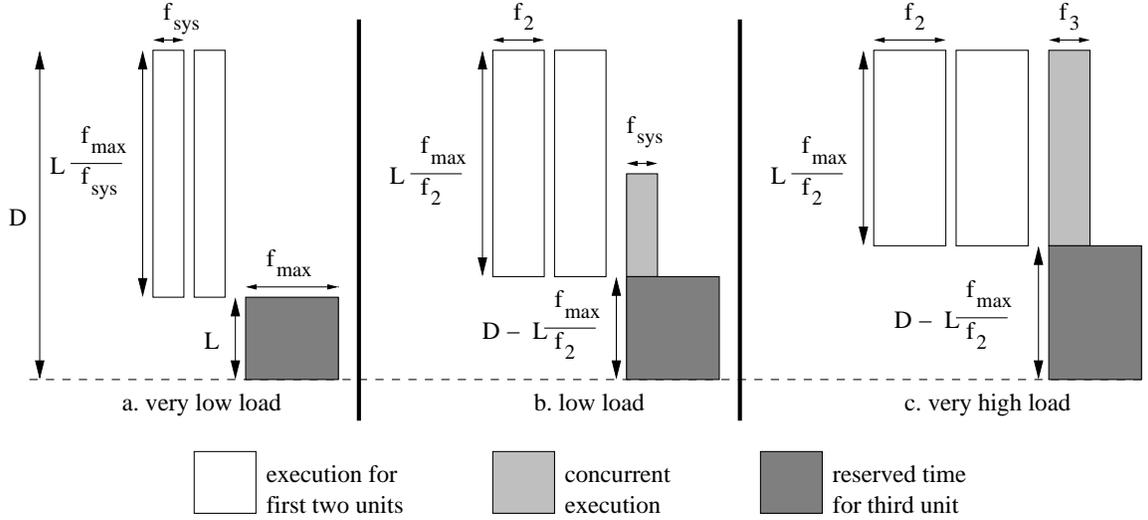
**Figure 1. Optimal speeds for OTMR under different loads: a. very low load ( $0 \leq \sigma \leq \frac{\kappa}{1+\kappa}$ ); b. low load ( $\frac{\kappa}{1+\kappa} < \sigma \leq \kappa$ ); c. very high load ( $\frac{1}{2-\kappa} < \sigma \leq 1$ ).**
