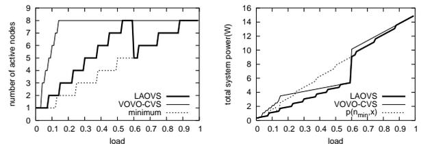
**Figure 5.** 8-node Intel XScale System without the frequencies 400MHz and 800MHz (theoretical results)
