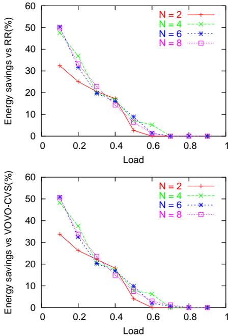
**Figure 6.** Energy savings of LAOVS as a function of load, compared to RR (top) and VOVO-CVS (bottom)
