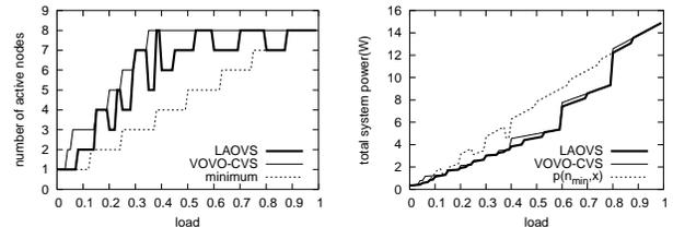
**Figure 4.** Intel XScale System with 8 nodes (theoretical results)
