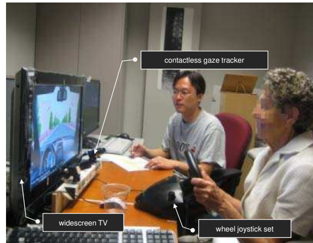
Figure 3. Experiment test-bed incorporated with a driving simulator with wheel joystick set and contactless gaze tracker.
