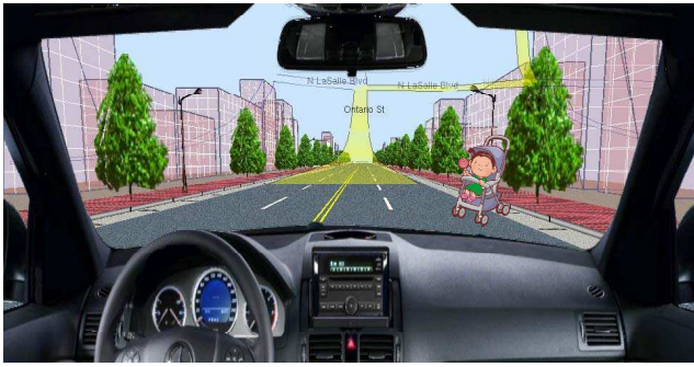
Figure 1. Screenshot of the simulated windshield-based 2.5 dimensional in-vehicle navigation display system.
