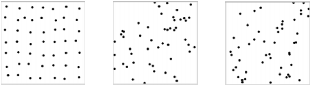
Figure 4.1: Snapshots of nodes' positions, generated by ad-hockey at 0, 100, 200 simulation seconds. The dots represent the nodes in the 1000m x 1000m simulation field. Number of nodes is 50 and node speed is 10 m/s.
